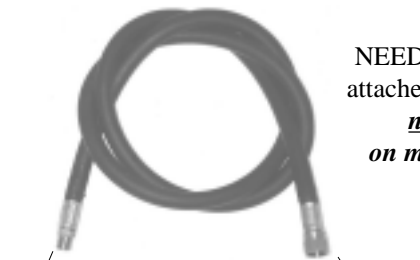
HOSE 1/4" MPT on one end attaches to needle valve or regulator 3/8" swivel flare on other end attaches to fitting on cooker
